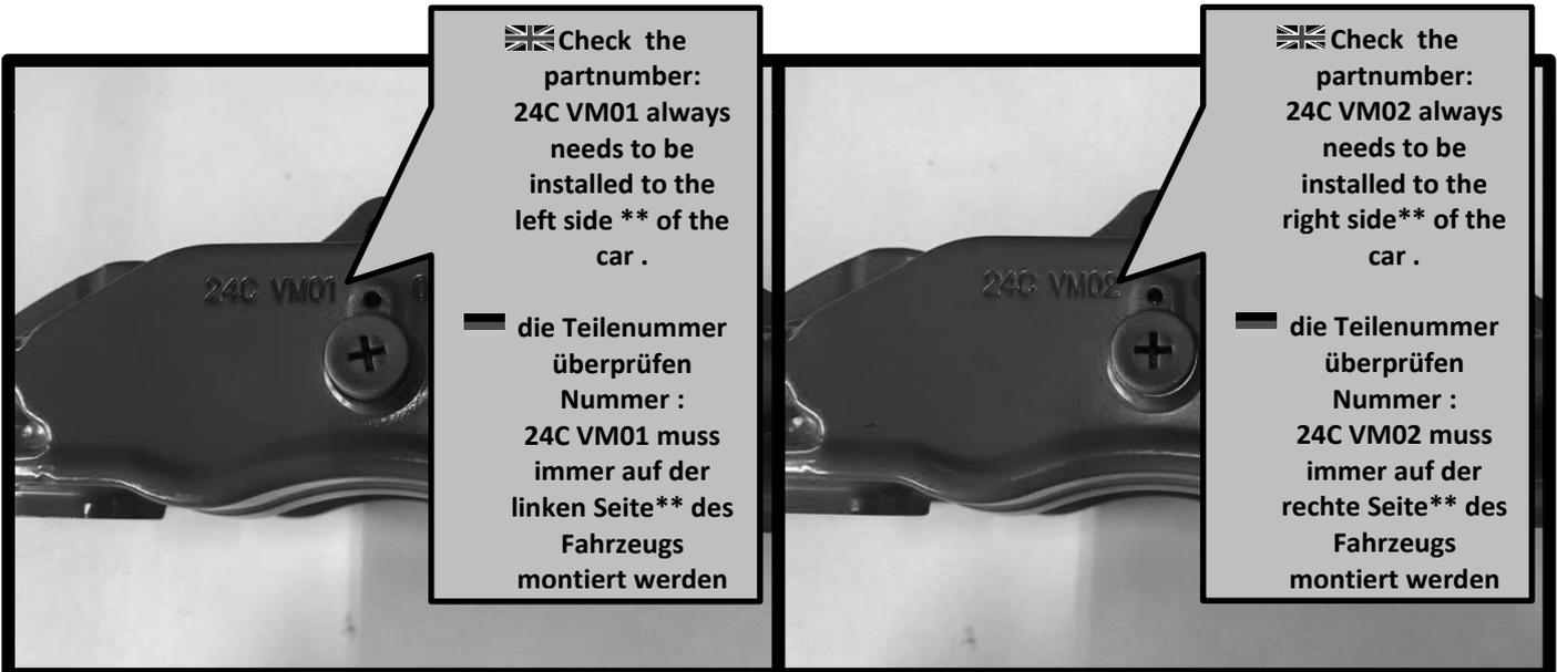
🇬🇧 Bleeding screws : always go on top of V-Maxx Autosport brake-caliper
