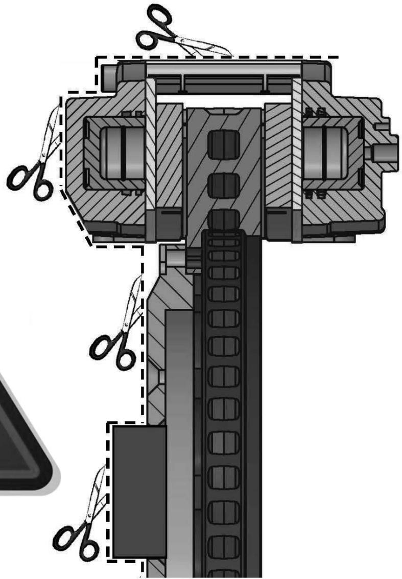
Please check clearance between the V-MAXX Big Brake Kit and your wheels the fitment of your wheels before installing ,using our wheel-fitment template.
